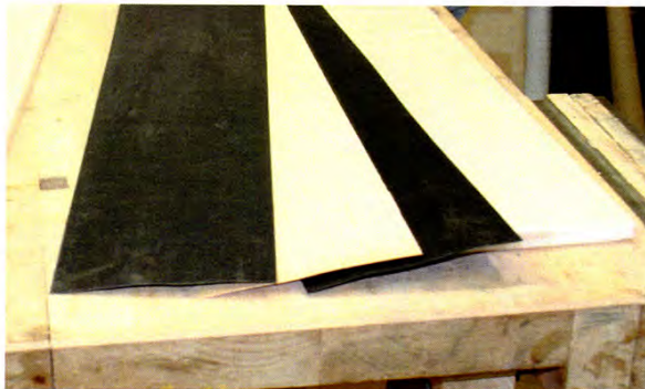
Fig. 5 Black and light veneers ready for laminating
