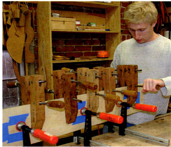
Fig. 18 Clamping sandwich together, caution should be taken not to shift the lamination causing gaps between chevrons
