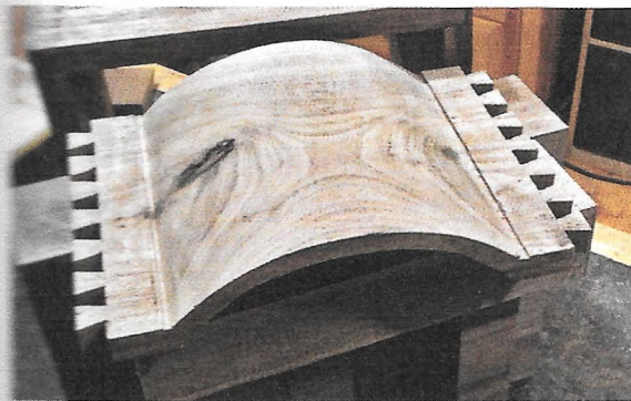
The top joints are completed and dry fit to the sides before working on the dovetail joints for the bottom.
