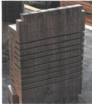
The initial cuts for the tails on the top were made using the bandsaw.
