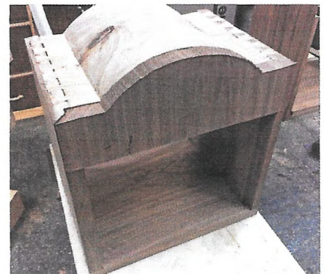
A dry fit of the carcass including the front top rail as it is fitted into its mitered seats in the case sides.
