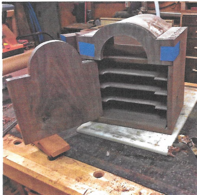
Behind the door the horizontal partitions carry the drawers. The fronts are cut back to provide room for the drawer knobs.
