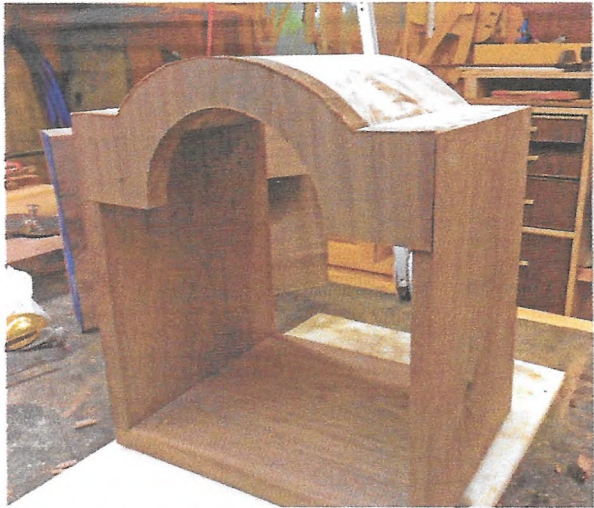
The final step to complete the top rail is to cut the inner radius. With these parts fit, the case is taken apart to add dados for the partitions.
