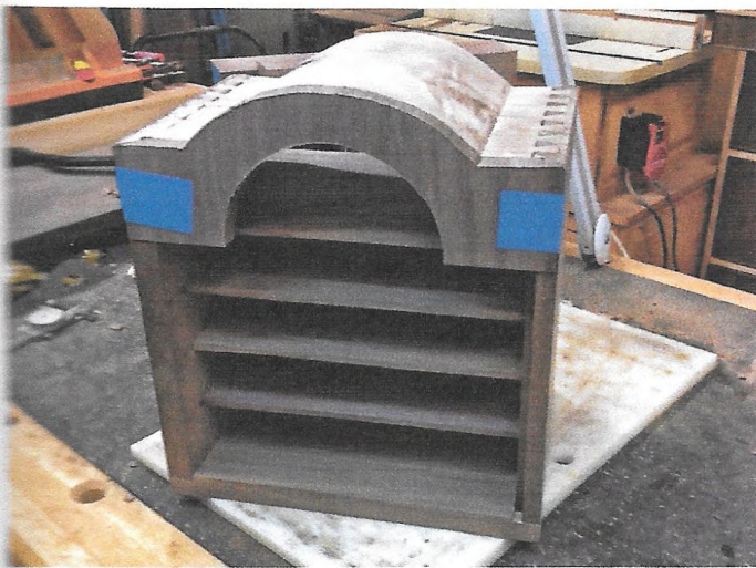
Dry fit seen from the front. The front edges of the partitions will be notched in the corners to cover the ends of the dados in the case sides.
