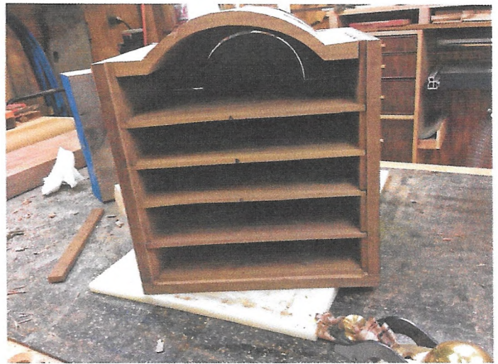
At the back the partitions and the arched case top end at the rabbet cut to accommodate the ship-lapped back boards.
