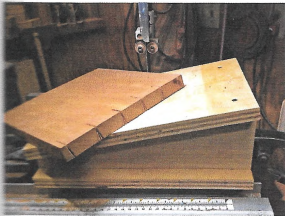
The pins are cut on the bandsaw using an angled jig. After making the cuts in one direction the jig is reversed to cut the other way.
